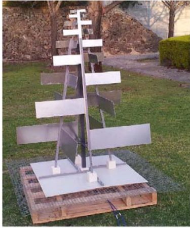
Cambridge University Log Periodic (wide-band) Prototype array element
