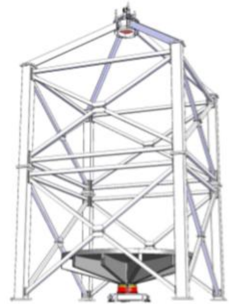
Figure 1. Left panel: Panoramic view of the ILMT site. The 1.3-m DFOT and the 4-m ILMT are in the middle and right side, respectively in this image. Right panel: Major components of the ILMT. Here, the container is gray, the air bearing is red, the three-point mount (white) sits below the air bearing and the vertical steel frames (white) hold the corrector and the CCD camera at the top. The tentative size and other parameters of the telescope are listed in Table 1. Note the nice view on the Himalayan chain in the background of the left photograph.
