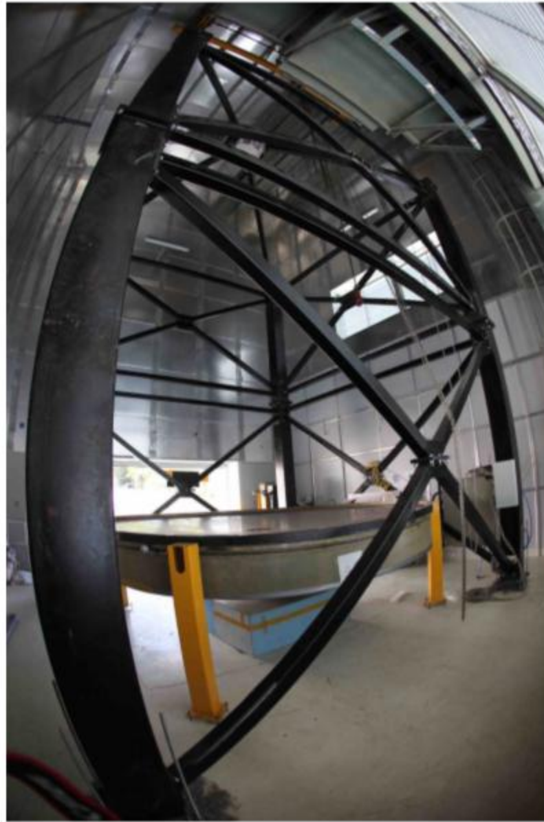
Figure 2. Fish eye view of the present status of the ILMT. To protect from the dust, the air bearing and the three-point mount are covered with a wooden box (blue colour). Four safety pillars (yellow colour) are also visible near the parabolic container to prevent any mercury spill.
