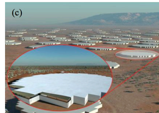
Dishes, sparse aperture arrays, and dense aperture arrays, Garrett+ 10, a concept design for SKA Phase 1
